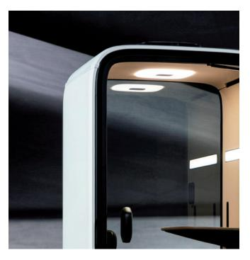
Framery One's powder-coated exterior panels are made from deepdrawn steel. Matt black structures made from aluminum and steel create the framing, and sound-control laminated glass finish the structural support. Replaceable interior paneling is made from PET sound-absorbing material. Anti-static, stain resistant low-loop pile carpeting covers the flooring.
